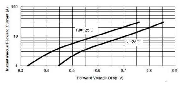
Fig.3-Typical Instantaneous Forward Voltage Characteristics
